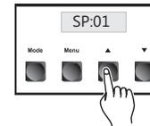
4. **Setting your desired Chase Speed:** In this mode, you can adjust the program chase speed. Use the "UP" and "DOWN" arrow buttons to adjust the chase speed from 01 thru 99. A set value of 99 will give you the fastest chase speed (approx. 1/10th of a second). While a set value of 01 will give you the slowest chase speed (once every 30 second.).
